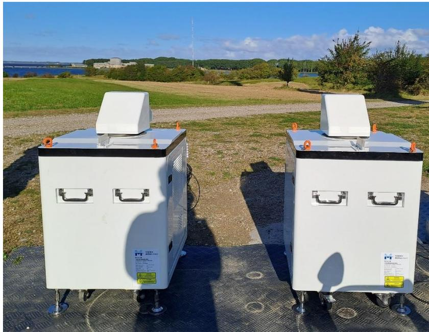
**Figure 4.1.1 Lidar installation pad with view towards reference mast. Unit 27 is installed on the right and unit 28 on the left.**
