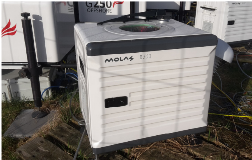
Figure 2.4: The RSD under test installed next to the met tower.
